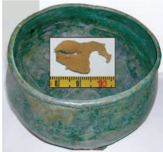
Figure 5. Original washbowl artefact and its fragment analyzed by PGAA, with reference to the sample No. 8.
